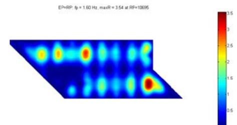
Figure 10: Vibration response simulations using first-principles approaches and published design guidance on footfall forces. R=1 denotes frequency weighted RMS response of 0.005/sec<sup>2</sup>.
