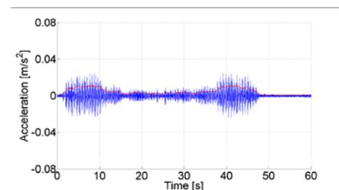
Figure 12: Floor response for walking at 1.58Hz (top) without AVC and (below) with AVC engaged.
