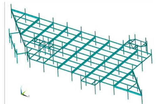
Figure 4: Beams and columns of initial FE model
