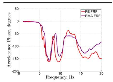
Figure 9: Matching of EMA and FEA frequency response functions for TP04, using updated FEA model.
