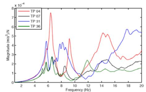
Figure 6: Driving point mobilities (accelerance or inertance values)
